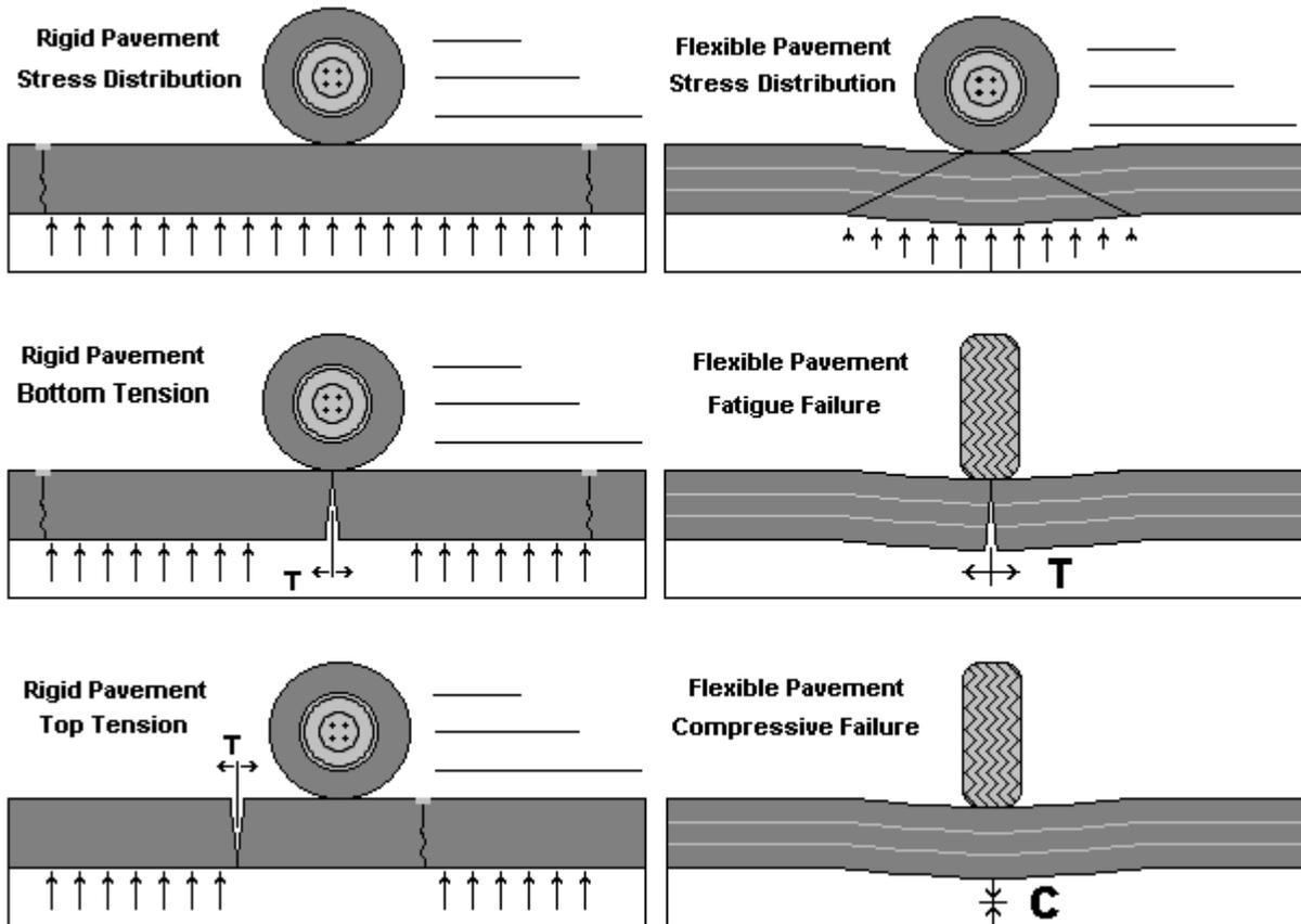
Figure 1. Pavement failure.
