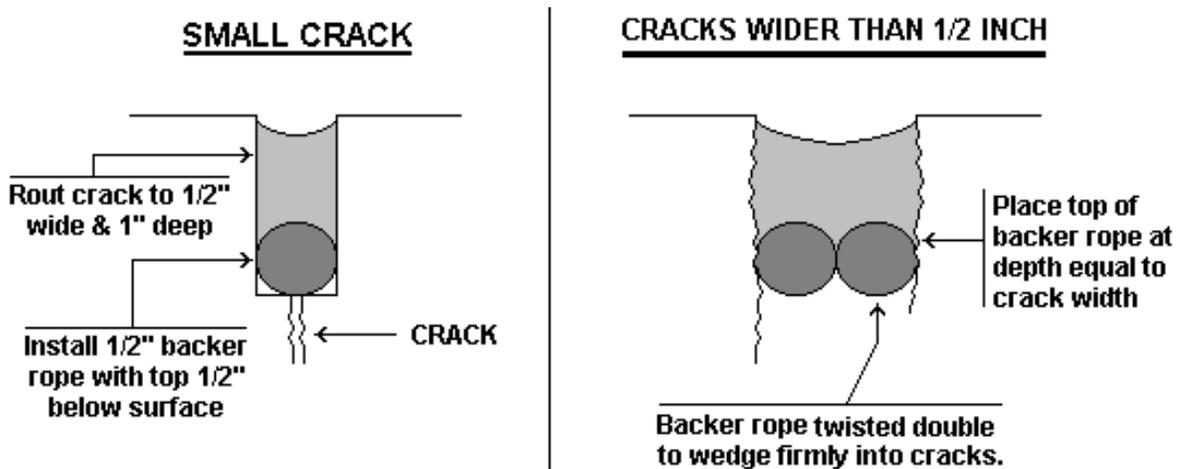
Figure 2. Crack sealing.
